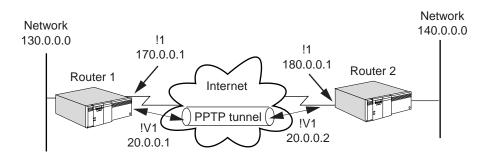
On router 1, set up the tunnel from 170.0.0.1 to 180.0.0.1 by following these steps.
